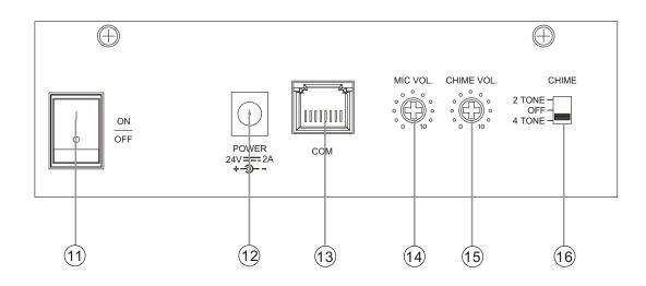
**11. POWER SWITCH.** The paging console is powered from the matrix through CAT5 cable.Power on when power switch is placed at on position, and power off when power switch is placed at off position.
