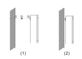
(1) Select the screw must suitable for the back side fixed hole size, twist the screw hole in the wall,put the screw into the opening hole site,fix the speaker in the screw.
