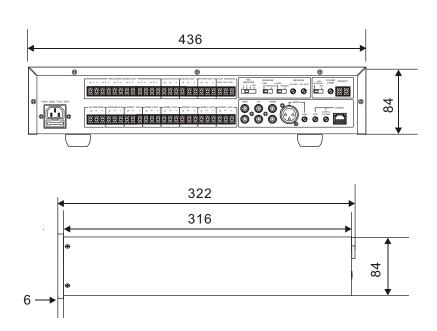
Keep the unit's all sides over 10 cm away from objects that may obstruct air flow to prevent the unit's internal temperature rise.
