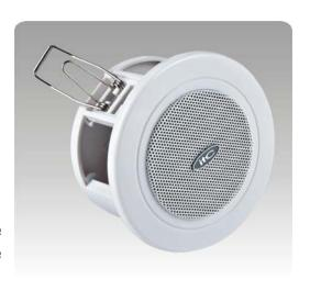
The built-in 3" speaker driver is designed of wide frequency response 120-20kHz, the multiple power taps 3W & 6W are helpful for different applications varies from room size and ambient noise surroundings. The metal grille and ABS baffle are painted in attractive RAL9016 white color. Its spring clamp makes the easy and secure installation.
