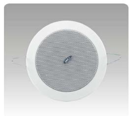
The built-in 4" water-resistant speaker driver is designed of wide frequency response 90-18kHz, the multiple power taps 3W & 6W are helpful for different applications varies from room size and ambient noise surroundings. The metal grille and metal baffle are painted in attractive white color. Its spring clamp makes the easy and secure installation.
