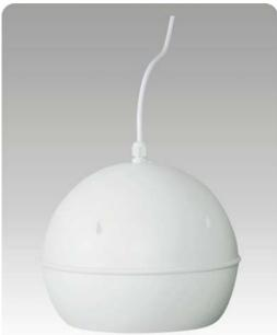
The built-in 5" full range speaker driver is designed of wide frequency response 130-14kHz, the various power output 1.5W, 3W & 6W could meet different applications varies from room size and ambient noise surroundings.
