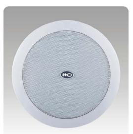
The built-in 5"+1.5" coaxial paper speaker driver is designed of wide frequency response 80-20kHz, the multiple power taps 0.75W, 1.5W, 3W & 6W are helpful for different applications varies from room size and ambient noise surroundings. The metal grille and ABS baffle are painted in attractive white color. Its flush mount type makes the easy and secure installation.
