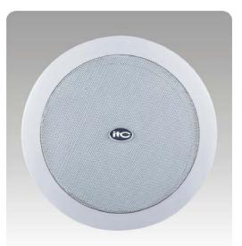
The built-in 8"+1.5" coaxial paper speaker driver is designed of wide frequency response 80-20kHz, the multiple power taps 1.87W, 3.75W, 7.5W & 15W are helpful for different applications varies from room size and ambient noise surroundings. The metal grille and ABS baffle are painted in attractive white color. Its flush mount type makes the easy and secure installation.
