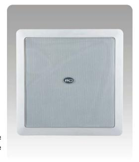
The built-in 8" speaker driver is designed of wide frequency response 80-20kHz, the multiple power taps 1.87W, 3.75W, 7.5W & 15W are helpful for different applications varies from room size and ambient noise surroundings. The metal grille and ABS baffle are painted in attractive white color. Its flush mount ears make the easy and secure installation.
