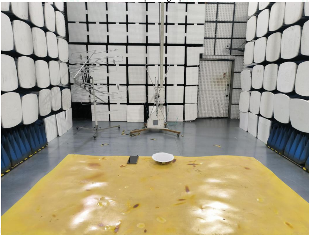
Test Setup Photo of Radiated Measurement (30MHz~1GHz)
