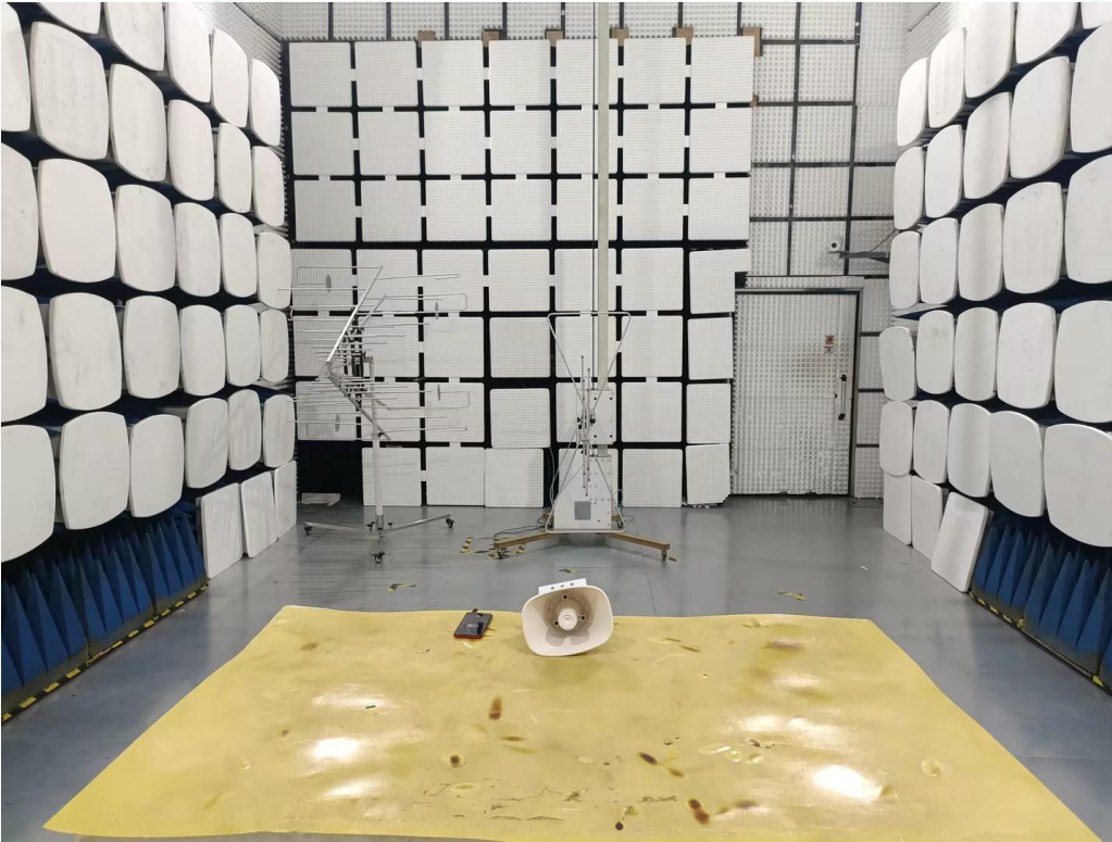
Test Setup Photo of Radiated Measurement (30MHz~1GHz)
