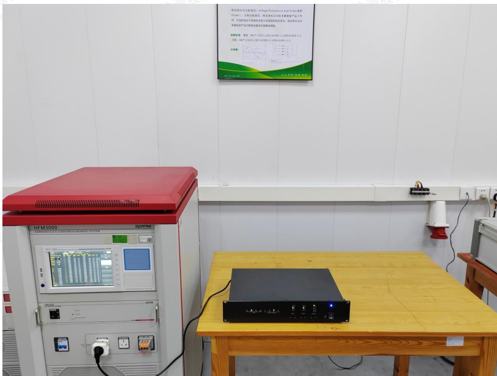
Test Setup Photo of Harmonic & Flicker Measurement
