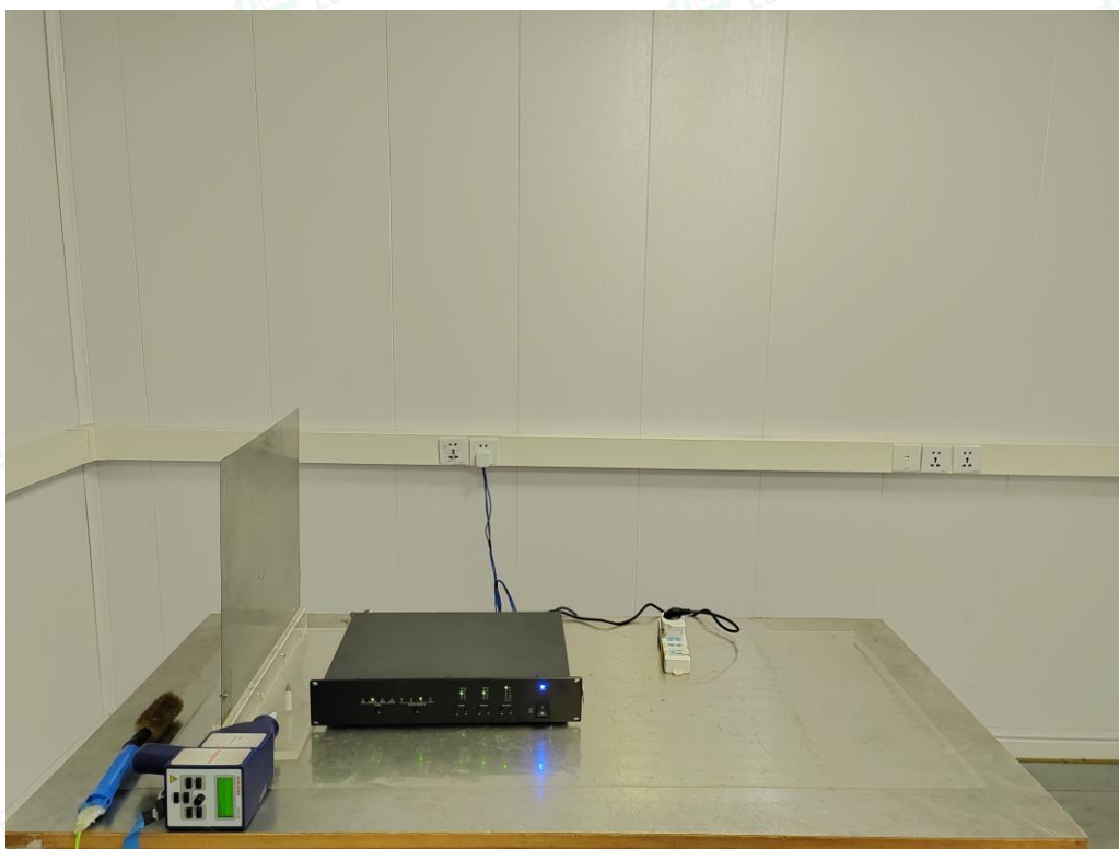
Test Setup Photo of Electrostatic Discharge Test
