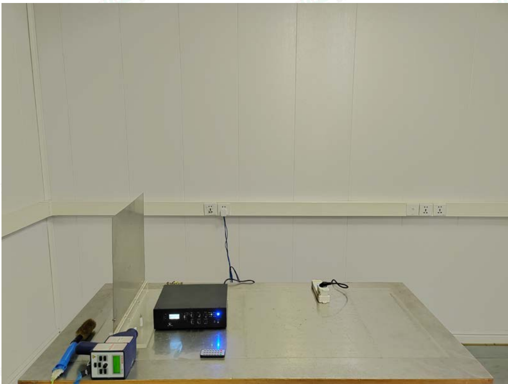
Test Setup Photo of Electrostatic Discharge Test
