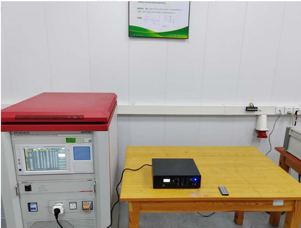
Test Setup Photo of Harmonic & Flicker Measurement
